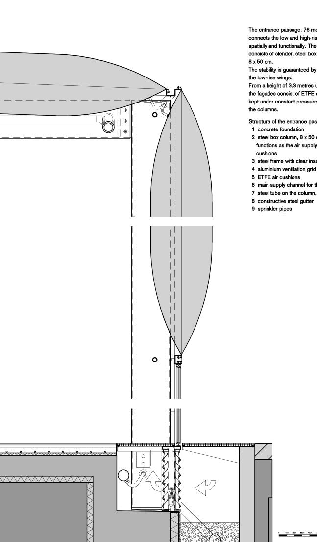
The entrance passage, 76 metres in lenght, connects the low and high-rise sections both spatially and functionally. The supporting structure consists of slender, steel box columns measuring
