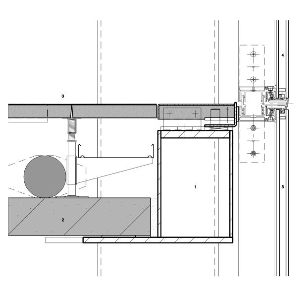
Exterior façade of offices: detail of floor edging and horizontal detail
